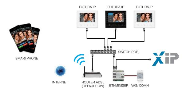
Installation diagram with separate power supply
